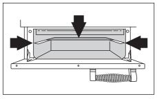
After placing your food on the broiler pan grid, slide the broiler pan onto the side supports just below the elements. Make sure it is pushed right in and touches the backstop.
